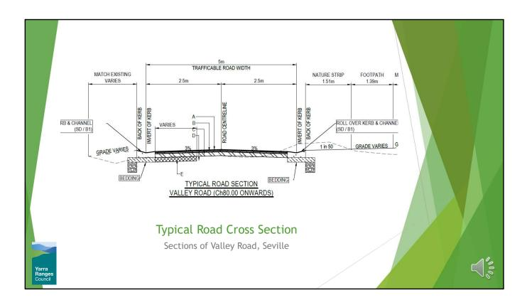
Here is a picture <u>Valley Road's</u> cross section with asphalt pavement and rollover kerb on either side.
