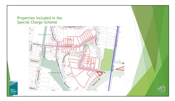
This map shows the extent of the scheme with **53** Properties involved highlighted in red. The extent of works is for **737 metres** of road to be constructed.
