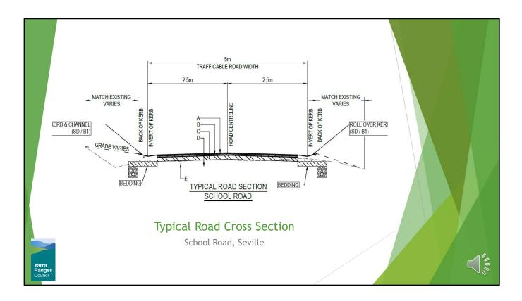
Here is a picture <u>School Road's</u> cross section with asphalt pavement and rollover kerb on either side.
